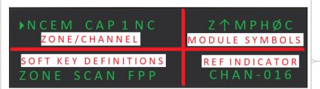
The screen can be divided into four separate area, each with a specific function.
