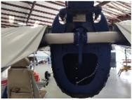
Wig-Wag on the landing lights are good; on the elevator it's bad. The Cessna elevator is actually two halves which join under the tail cone. They are each riveted to a bearing which allows easy travel. If there is play (one can move up, while the other down), the rivets are working loose.
