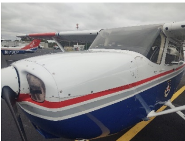
N908CP (FLO) had its' cowling, ailerons and a flap stripped and repainted during its recent 100-hour/annual inspection.
