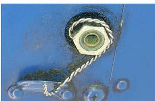
(Left) Fuel drain in center under cowling serving fuel selector valve: Won't drain much if fuel selector set to 'off.' (Right) Drain for gas-collator (on old & new Cessnas. Drains until the Gascolator is empty.
