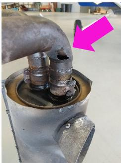
(Left) N99832’s Exhaust pipe hole. No wonder the aircraft sounded so loud. (Right) N963CP’s engine was removed & shipped out to Oklahoma for study. No one knows why it’s making noise & metal.
