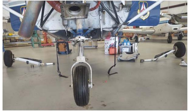
*Above left: We couldn’t top the FY18 trophy presented to Capt Herring, so we bottomed the award with two more tiers for FY17 & FY19. Above right – N4813C needed new main gear bushings which required removing the main landing gear.*
